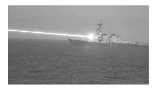
In this undated photo from fiscal 2024, the Preble fires its HELIOS system during weapons testing. (DOT&E)
